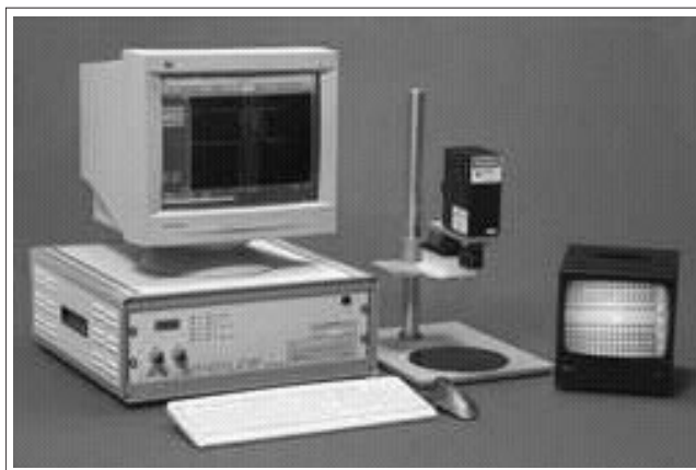
Fig. 4 Interferometric Endpoint Detector and Thin Film Monitor, DigiLem Series
