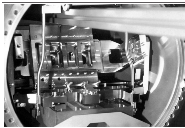
Fig. 2 Inner View of Eagle Off Plane Monochromator Chamber Installed at LURE (France)
