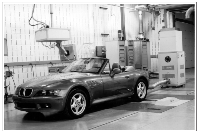
Fig.4 HAD Test Cell Showing Vehicle on Dyno with MEXA-7000 Instruments in the Background
