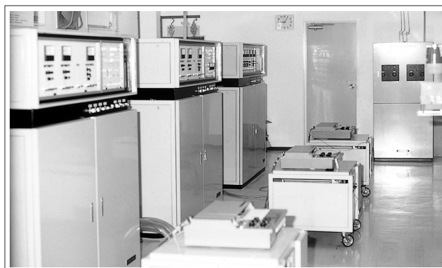
Fig.2 SGGs-1 Standard Gas Generator for Pollution Meter Calibration
