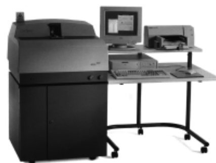
Fig.4 Multi-Dispersive X-ray fluorescence element analyzer MDX-1000
