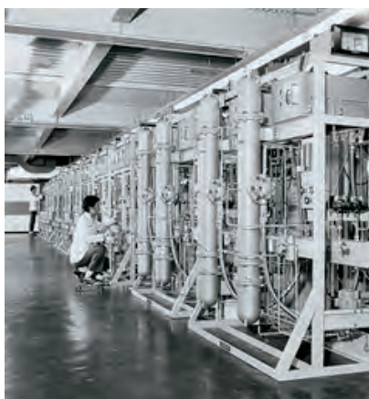
Figure 10 10 ppm CO MEAS. in NH 3 GAS PRODUCTION PROCESS, TIA-1 NDIR (1 m CELL)
