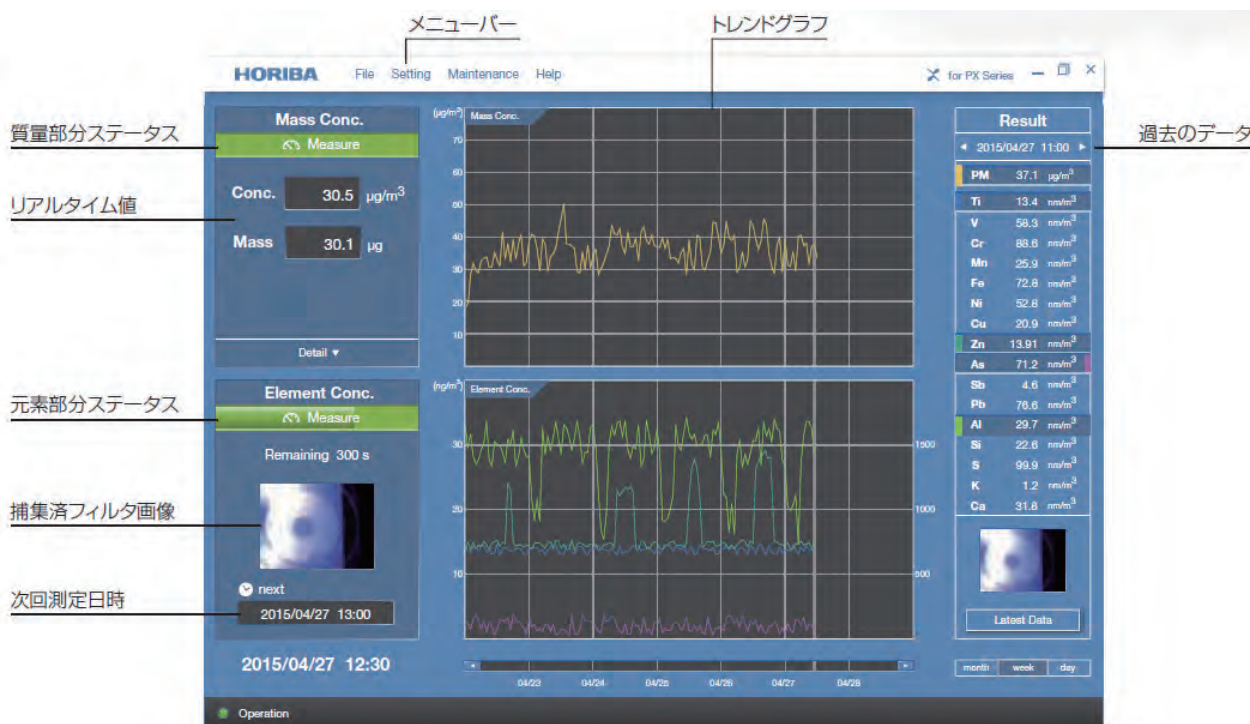
Figure 2 Screen of measurement monitoring
