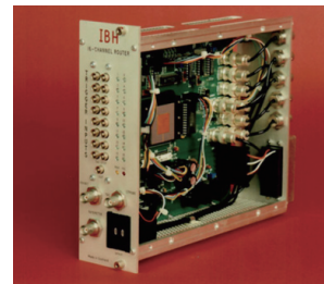
Figure 2 Model 5000W SAFE and its 16 channel TCSPC multiplexing module.
