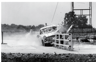
Figure 6 Crash testing on the High Energy Facility
