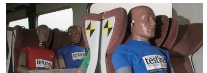
Figure 16 Crash test dummies used in full-scale rail crash testing
