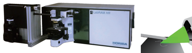
Figure 17 LabRAM HR-AFM coupling system The right picture shows the configuration of incident laser-radiation with 60 degrees angle at samples.
