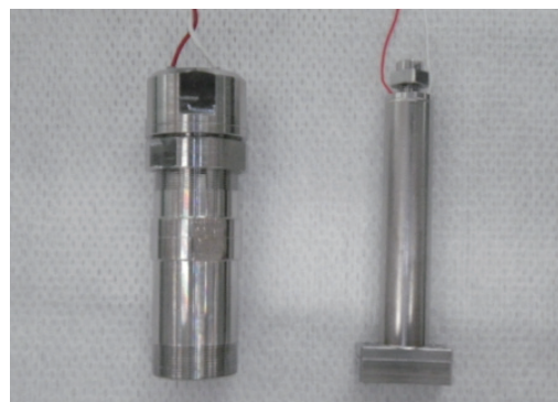
Figure 15 (Left)Previous machined case (Right)New small case
