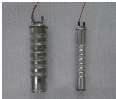
Figure 3 (Left)Standard bellows (Right)Small bellows
