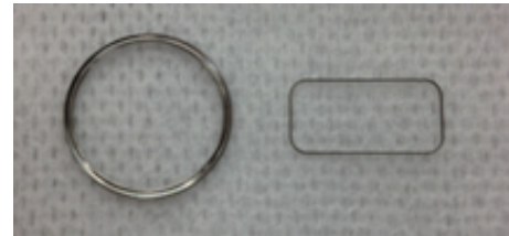
Figure 12 (Left)Circular shape gasket (Right)Rectangle shape gasket
