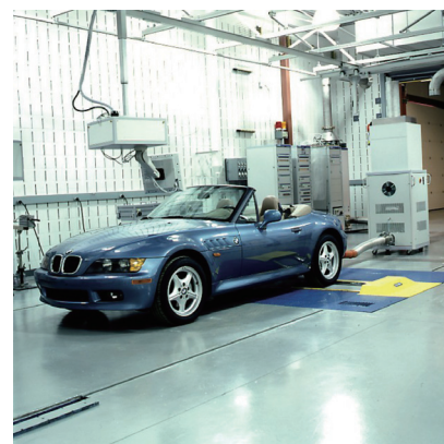
Figure 3 Example of Vehicle Test Cell with a Chassis Dynamometer
