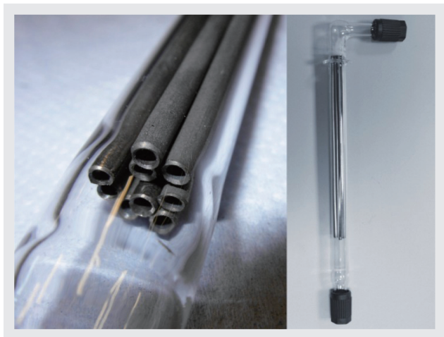
Figure 6 Catalyst glass pipe close-up view placed in the oven. The glass pipe is filled with 9 tubes of stainless steel (7301 SS, 1.4301). Each tube has a diameter of 3 mm with void of 2 mm.
