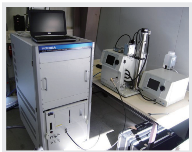
Figure 4 SMPS System with DMA and CPC
