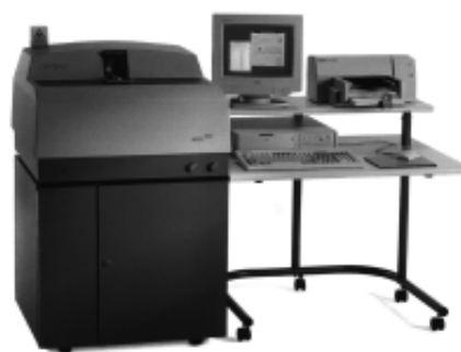
Fig.4 Multi-Dispersive X-ray fluorescence element analyzer MDX-1000
