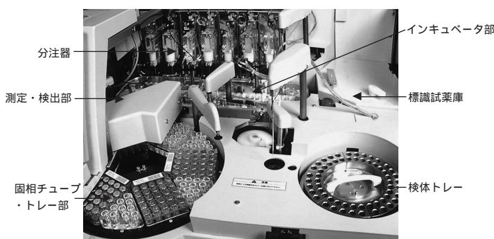
図3 反応・測定部 The reaction and measurement chamber
