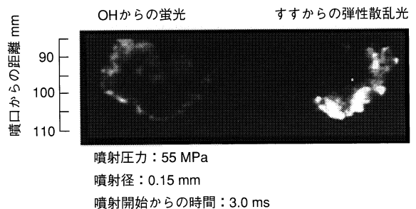
図4 火炎内のすすとOHの同時可視化画像 Images of LIF emission of OH and elastic scattering of soot in a flame taken simultaneously
