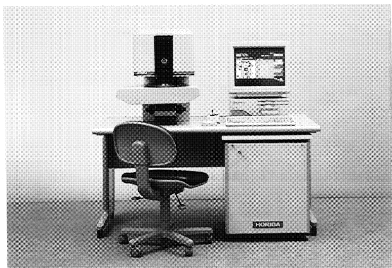
図1 卓上型X線分析顕微鏡 Outline of X-ray analytical microscope
