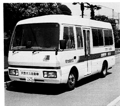
図3 小型バスを改造した環境測定車 Vehicle developed for measurement of the environment (reformed small-sized bus)
