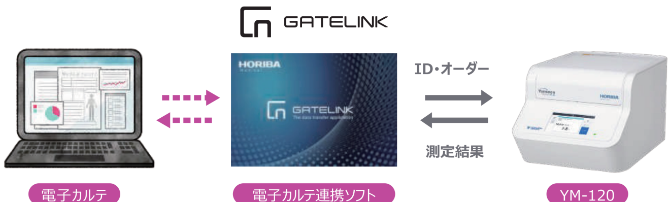
Figure 6 GATELINK connection configuration diagram
