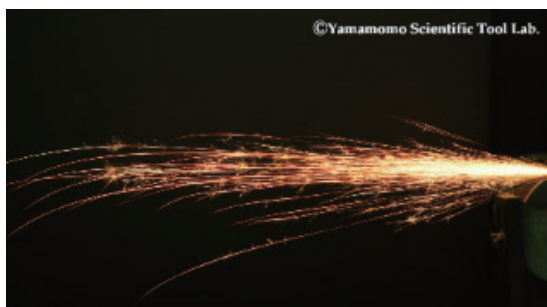
Figure 1 JIS G 0566(1980) Spark test method for steel.*
