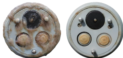
Figure 3 Effect of ultrasonic cleaning on Ammonium Probe: Without (left) and with (right) cleaner after 60 days. https://static.horiba.com/fileadmin/Horiba/Products/Water/Download/Brochures/HAE-T0257.pdf
