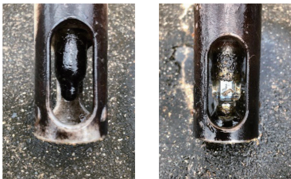
Figure 5 Without (left) and with (right) self-cleaning function after 3 months. https://www.horiba.com/int/water-liquid/products/other/self-cleaning-ph-electrode/
