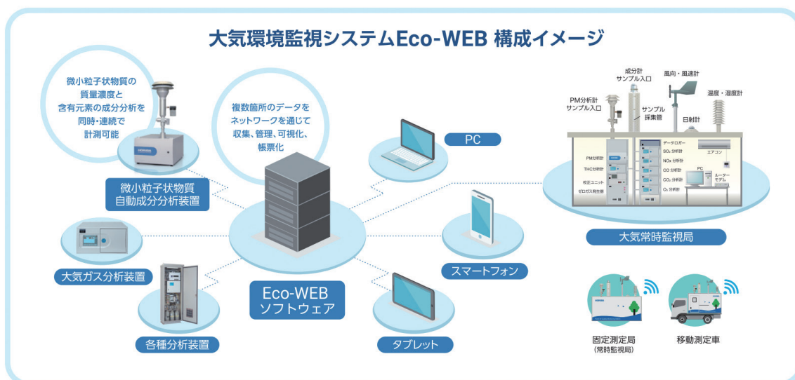
Figure 5 'Eco-WEB' Air Quality Monitoring System Configuration.
