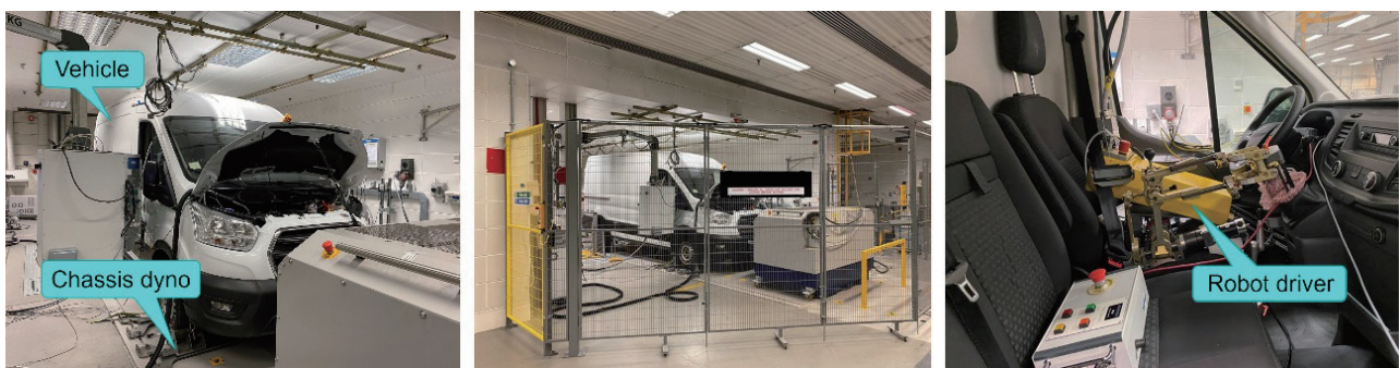
Figure 5 Vehicle and corresponding diesel engine tested at an OEM in the UK.
