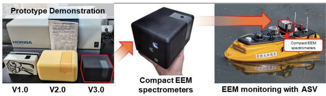
Figure 3 Homemade compact EEM spectrometers
