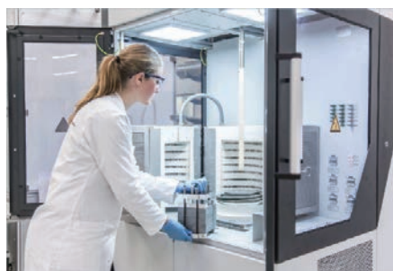
Figure 13 Evaluator C1000-HT SOFC Fuel Cell Test Station.
