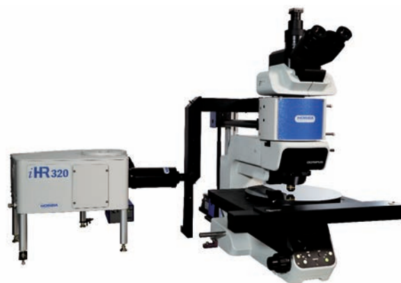
Figure 1 HORIBA multimodal, Standard Microscope Spectroscopy (SMS) system equipped with 12-inch wafer stage.
