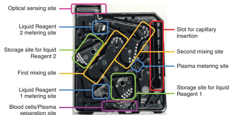
Figure 4 Functional sites of CRP reagent chip
