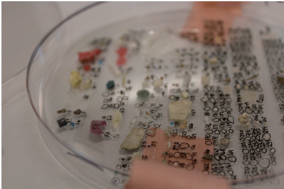
Figure 4 Examples of picked MP particles from a subset of a single experiment showing the large quantity and variation of particles that can be generated in MP analysis studies. Image reproduced by permission from the Rochman group.
