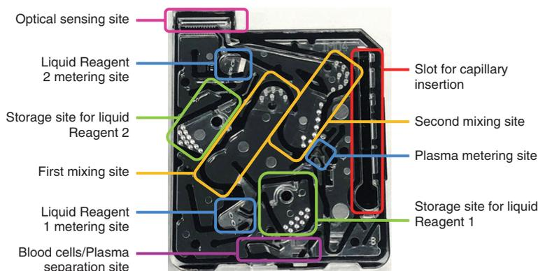
Figure 4 Functional sites of CRP reagent chip
