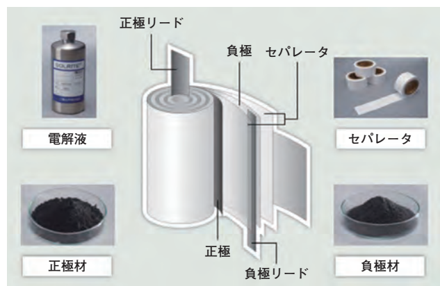
Figure 3 Main components and structure of lithium ion battery
