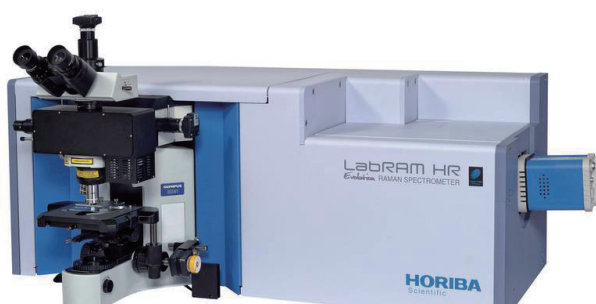
Figure 1 Confocal Raman Microscope LabRAM HR-Evolution
