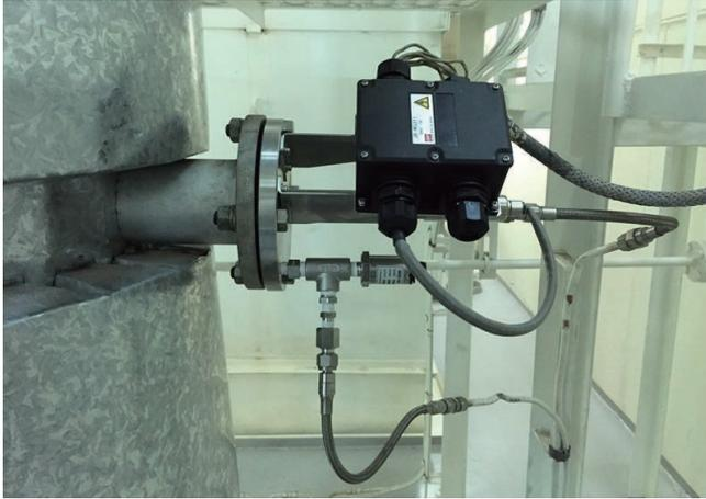
Figure 13 MEXA-820NO<sub>x</sub> arranged in the front and the rear of SCR
