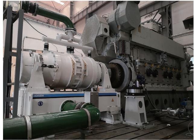
Figure 3 Engine test stand with hydraulic dynamometer and ship engine (Weichai Power, China)<sup>[5]</sup>
