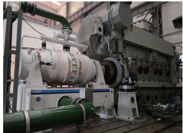
Figure 3 Engine test stand with hydraulic dynamometer and ship engine (Weichai Power, China) [5]
