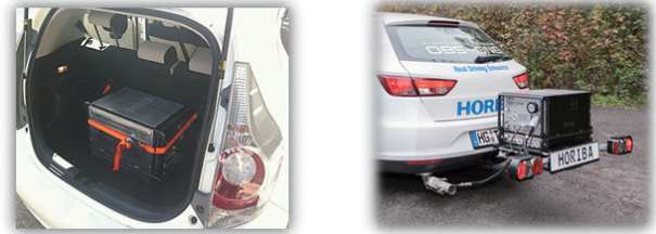
Figure 2 Installation of PEMS on the vehicle
