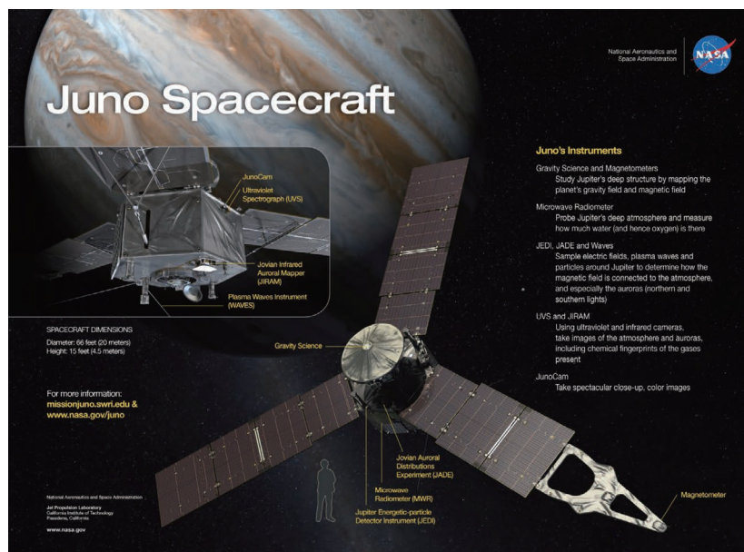
Figure 6 Picture of the JUNO Spacecraft including the HJY grating in the JIRAM instrument
