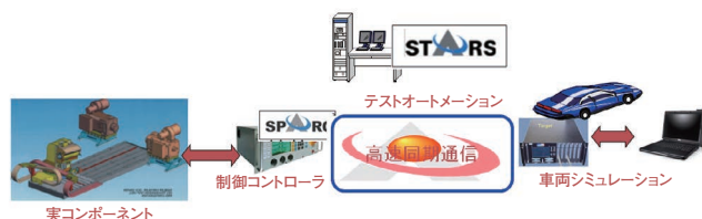
Figure 10 High Speed Synchronized Communication Image with HILS
