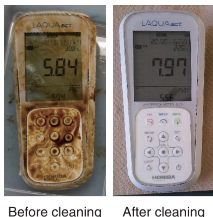
Figure 8 Outlook of LAQUAact(pH meter)with dipping into oil
