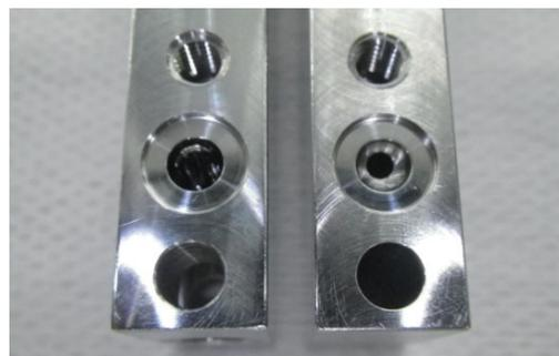
Figure 18 (Left)High flow block (Right)Standard block
