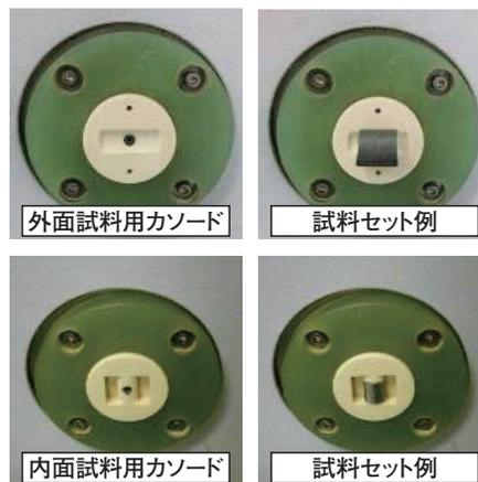
Figure 12 Tool for curved specimen
