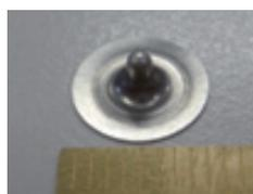
Figure 7 Pressed diaphragm
