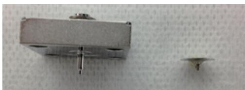
Figure 5 (Left)Standard Diaphragm (Right)Small Diaphragm
