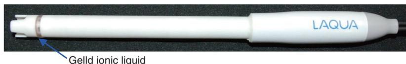
Figure 1 The picture of PUREIL electrode
