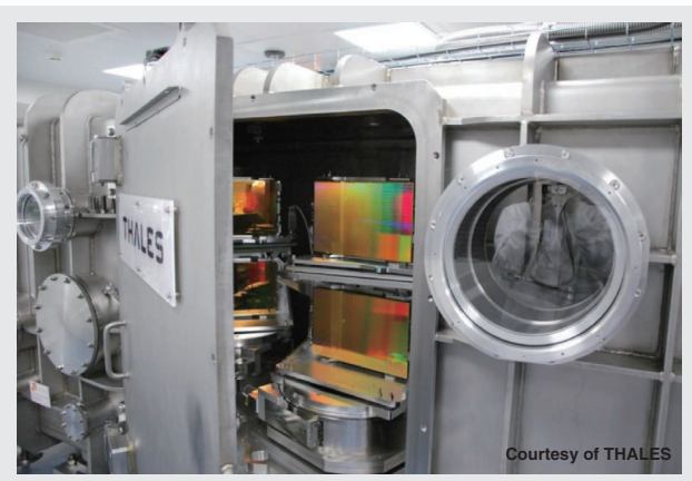
Figure 3 Pulse Compressor vacuum chamber with four HJY gold-coated diffraction gratings
