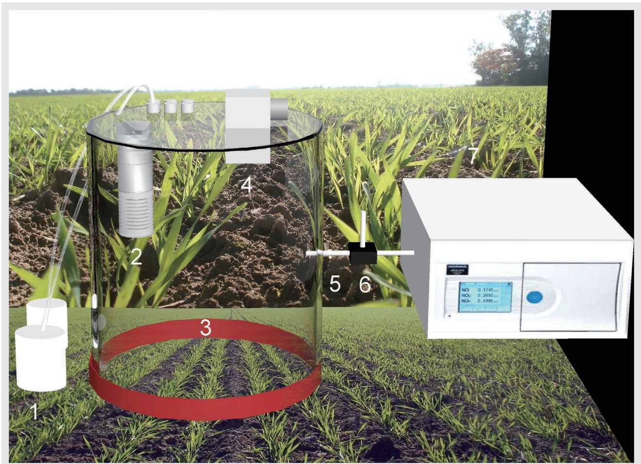
Figure 1 Measuring Setup to Analyse NO-Emissions from Soils. [5]
