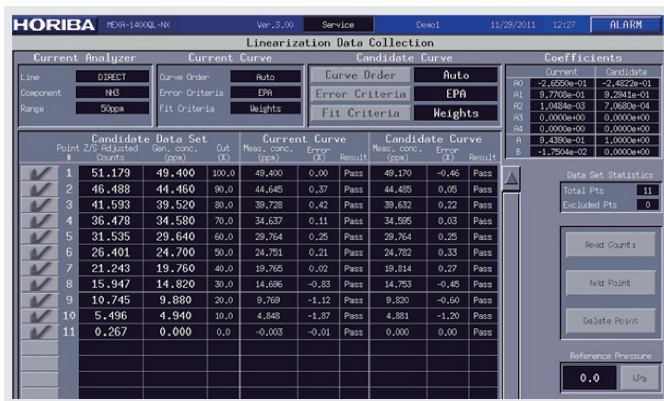
Figure 5 Screenshot showing typical results of a linearity test
