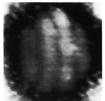
Fig.8(b) STM image of a C 60 molecule on the Si(111)7x7 surface shows the internal structure of the molecule 9) .
