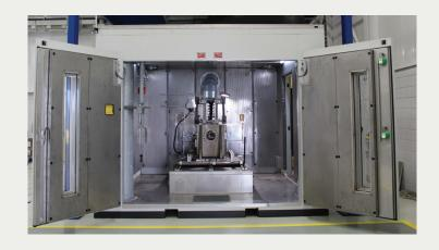
J2522) with brake torque and temperature measurements to quantify the loads the brake system is experiencing. A climatic system and insulated test chamber are equipped to perform climatic simulation, ranging from -40°C to +50°C and at 5 to 90% relative humidity. Customer specific test scripting and reporting are standard services that can be provided.
