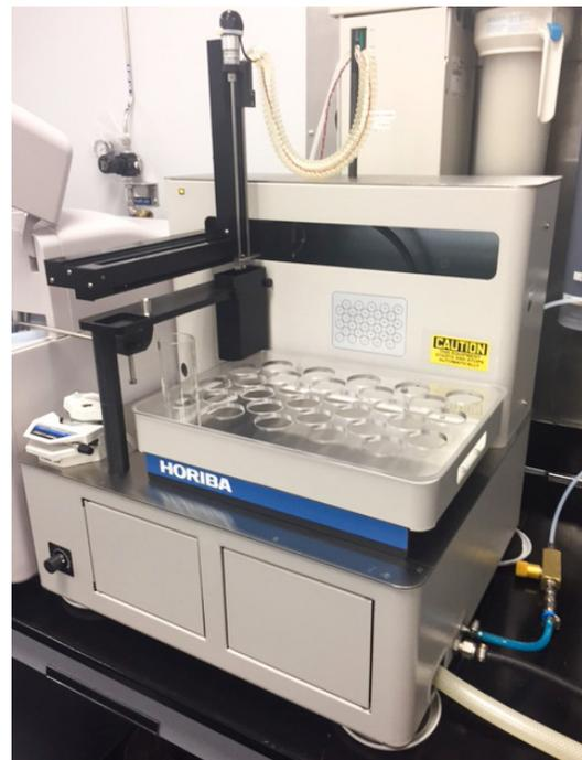
Figure 2. LA-960V2 Slurry AutoSampler
