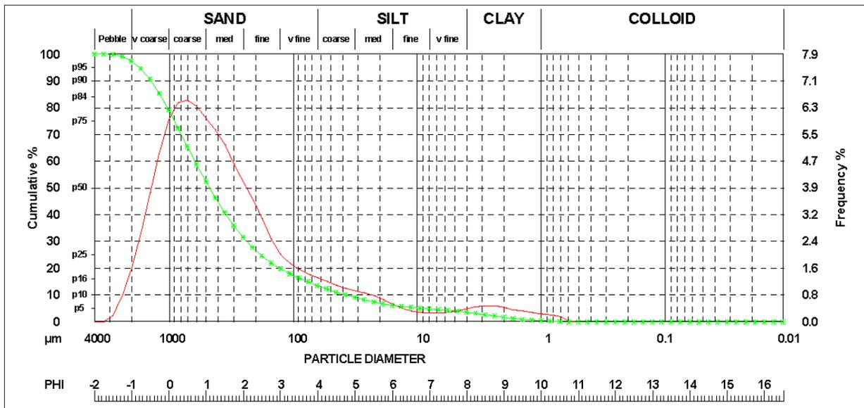
Figure 4. LA-960V2 Phi Scale Graph
