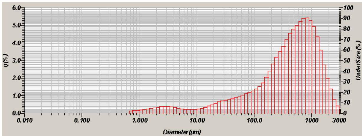
Figure 3. Lake sediment sample measured on the LA-960V2
