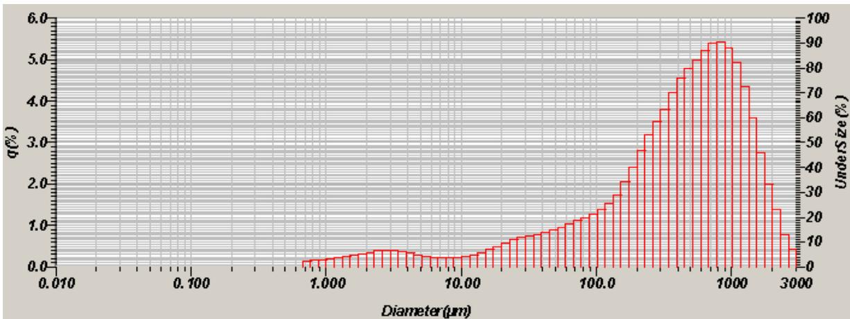
Fig. 3. Lake sediment sample measured on the LA-950
