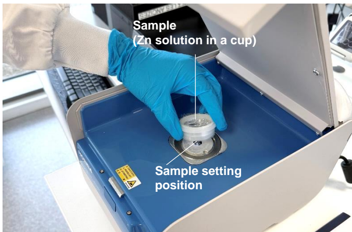
Figure 2. Sample setting inside the MESA-50 chamber.
