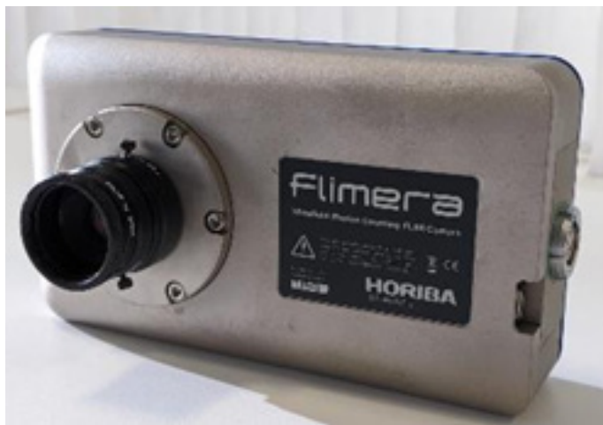
Figure 3. FLIMera equipped with a lens for macro imaging.
