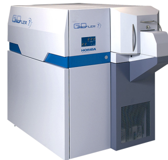
Figure 4. GD Profiler 2: 4 th generation of GD-OES
