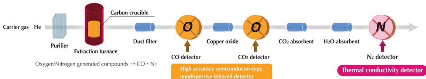
Figure 2: Gas flow diagram of the EMGA-820/EMGA-920
