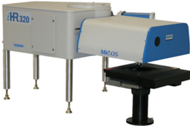
Fig. 2. Down-looking version of HORIBA MicOS with mapping stage.
