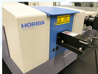
Figure 2: 980 nm DPSS laser mounted to the front of the Fluorolog-QM sample compartment.
