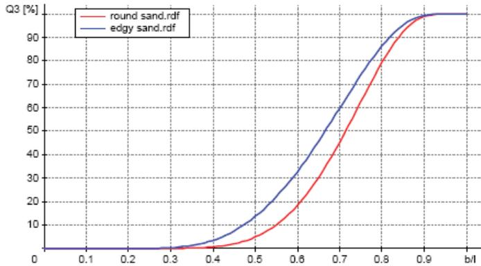
**Figure 1: CAMSIZER measurement of one edgy and one rounded sand type. The samples are similar in size, but parameters b/l and SPHT show the different shape. The round sand provides much better flowability if added to concrete as an aggregate.**
