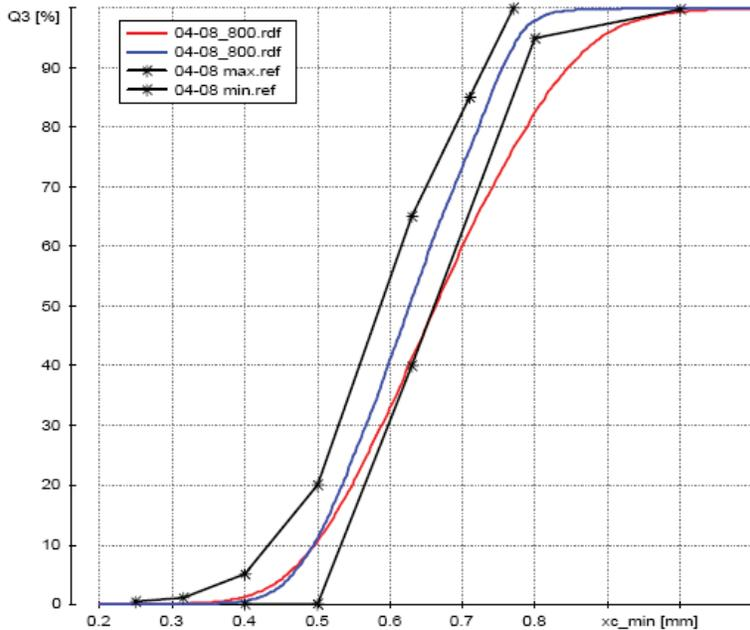
**Figure 2: Measurement of filter sand 0.4 – 0.8 mm.**
