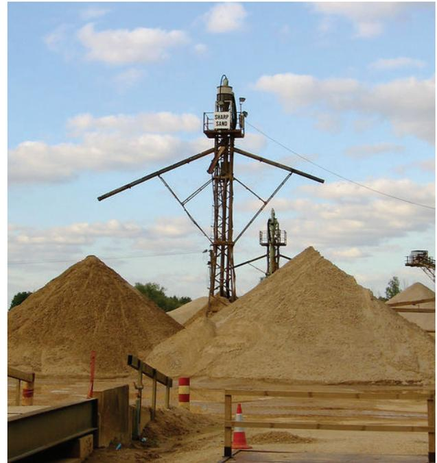
the material as well as the outer appearance. For 1 m<sup>3</sup> of “normal” concrete, 545 kg of aggregates 0-2 mm, 725 kg aggregates 2-8 mm and 545 kg aggregates 8-16 mm are needed (according to EN206 and DIN1045).
